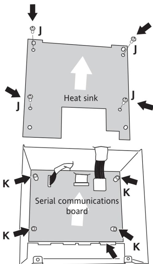
**10** To gain access to the serial communications board, the heat sink must first be removed, by undoing the four securing screws J, and lifting the heat sink out.
